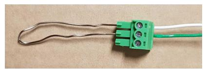
To demonstrate, if the lock mechanism is unengaged (unlocked) before you connect in the paperclip, it should be engaged (locked) after you connect the paperclip.
