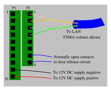
This image shows the connectors on the rear of the reader connect the LAN and the door circuit as shown.
