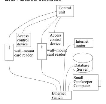
These RFID readers connect via ethernet LAN cables to a network switch instead of connecting directly to the server.
