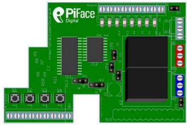
When wiring up the lock to the device, the default switch to use is the bottom one (blue in the diagram). Note that the top screw for the switch (relative to the orientation of the above image) is NC (normally closed), where as the bottom screw is NO (normally open).
