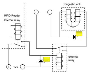
For locks that require power to lock you can stwitch locking current by putting a relay in series with the lock. Remember to fit diodes, failure to do so may lead to the RFID reader quitting.
